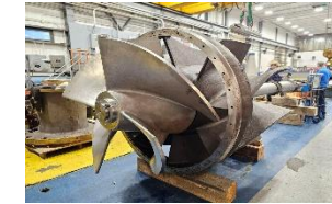
Pump under repair (coal)
